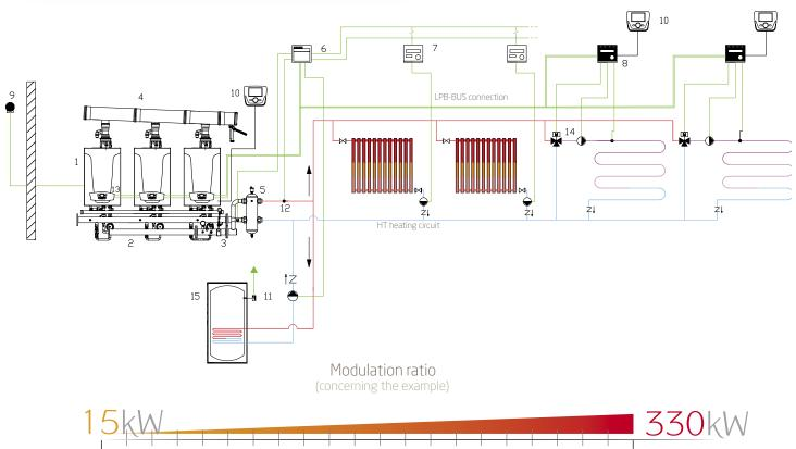
Cascade installation in a multi-dwelling building with CH and DHW production with centralized tank, indipendent zones, control with room thermostat.
